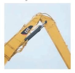
**Dual Stick Cylinders.** Provides excellent geometry for working close in to the machine or at full reach.
