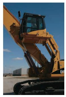
**Hydraulic Cab Riser.** Optional hydraulic cab riser provides up to 2.6 m (8'6") of additional operating height. There is easy access to the cab platform provided by handrails attached to the riser.
