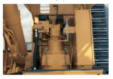
**Generator Set.** A 20 kW (26.8 hp) hydraulically driven generator set can power magnets up to 1.68 m (66") in diameter.
