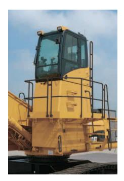
**Fixed Riser.** Cat® designed and built, 1.95 m (6'5") manual tilt cab riser provides for operating height with excellent visibility for loading and unloading processing equipment, trucks, and rail cars. Access to the cab is provided by a ladder to the platform extending around the cab riser. This platform allows for windshield cleaning. The cab riser can be manually tilted forward 90 degrees for shipping.
