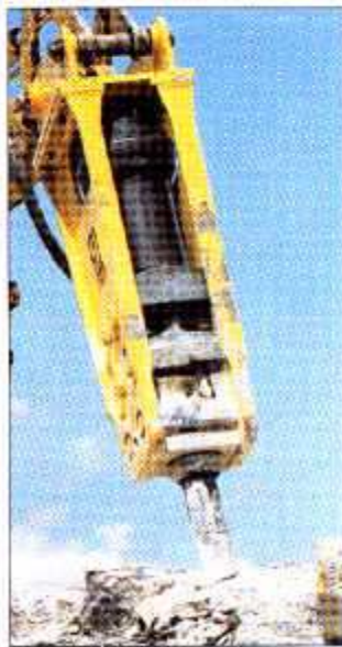
Break up concrete and handle other demolition work with a hydraulic hammer.
