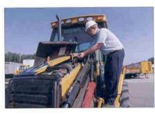
Flip-Open Hood. The flip-open hood opens easily and provides convenient access to all engine check points from the left side of the machine.
