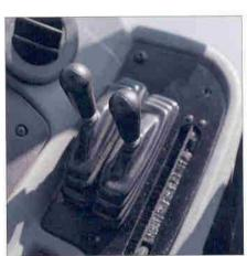
Pilot Operated Stablizer Controls. These provide low effort and fine modulation control. The stabilizer controls are within easy reach of the operator when operating the backhoe.
