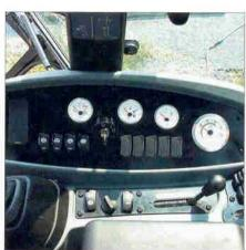
Machine Controls. Switches are relocated to operator level and the boom lock and pilot-operated stabilizer controls, which provide low effort and fine modulation, are within easy reach of the operator. New white-faced gauges are easy to read.
