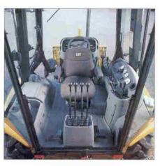
Utility Plus Cab. Includes two doors with opening glass, a radio ready headliner, 12-volt power supply, a left side storage console with drink holders,
