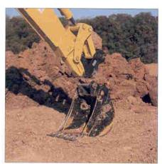
Quick Couplers. Allow for quick attachment of buckets and other work tools. The D-Series High Rotation pin grabber design and a C-Series compatible pin grabber allow buckets to be changed without removing the bucket pin. Other manufacturers' buckets can be coupled with a pin puller coupler, one for Case and D-Series buckets and one for John Deere and D-Series buckets. D-Series Quick Couplers are painted black for easy identification.
