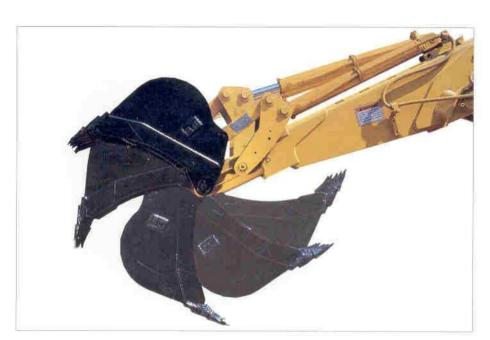
High Rotation Backhoe Linkage. Single pin bucket linkage contributes to bestin-class rotation of 205 degrees for all applications, elminating the need to change pin position when moving from loading trucks to vertical wall trenching.
