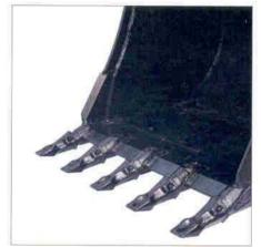
Diagonal Retention System. Bucket teeth are attached with diagonal pins rather than horizontal pins for easy exchange of bucket teeth. The adapters are stronger as a result of this diagonal pinning and additional wear material on the bucket teeth increases durability.
