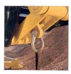
**Lift Eye.** An integral lifting eye is a standard feature of the bucket linkage.
