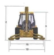
Dimensions and performance specifications shown are for machines equipped with 11L x 16 (10 PR) front tires, 19.5 x 24 (10 PR) rear tires, ROPS canopy, standard stick with 24-inch standard-duty bucket, and 1.0 yd\* loader bucket and standard equipment unless otherwise specified.
