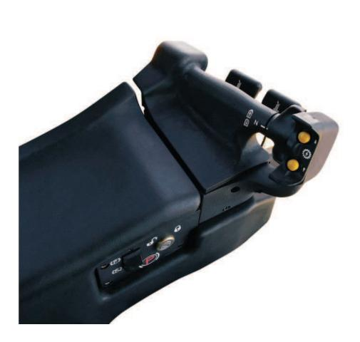
**Three-Speed Forward/Reverse Gear Selection.** Three-speed forward/reverse gear selection is achieved simply by pressing the yellow speed selection buttons. These buttons are integrated into the Finger Tip Control group. • Automatic shifting features and reduced lever efforts for easier upshift and downshift, increased operator comfort, reduced fatigue, and precise control.
