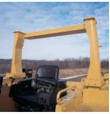
**Optional Roll Over Protective Structure.** Provides for increased operator protection.
