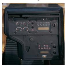
**Dash.** The instrument panel, with easy to read analog gauges and warning lamps, keeps the operator aware of any potential problems. All gauges and readouts are easily visible in direct sunlight. Auto-shift and Auto-kickdown controls are located within easy reach of the operator. New footpads keep the operator stable and comfortable during side slope applications.
