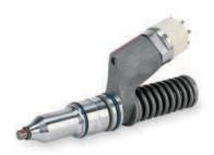
**Electronic Unit Injector (EUI).** The mechanically actuated, electronically controlled unit injector combines an electronic actuator, pump assembly and nozzle into a single, compact unit for reliability and durability. The 3176C fuel system has been tested in thousands of engines in some of the most demanding applications and environments around the world.
