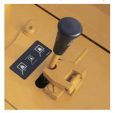
**Counterweight Control.** Adjusts the position of the counterweight for added machine stability.
