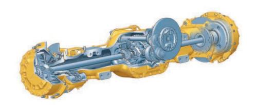
**Parking Brake.** The parking brake has been moved from the transmission to the center axle. This new design delivers higher heat capacity and abuse resistance.
