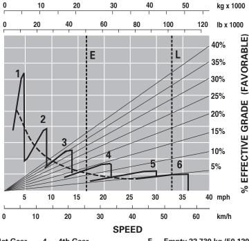
1 — 1st Gear 4 — 4th Gear 2 - 2nd Gear 5 — 5th Gear 3 - 3rd Gear 6 - 6th Gear E — Empty 22 730 kg (50,120 lb) L — Loaded 46 320 kg (102,136 lb)
