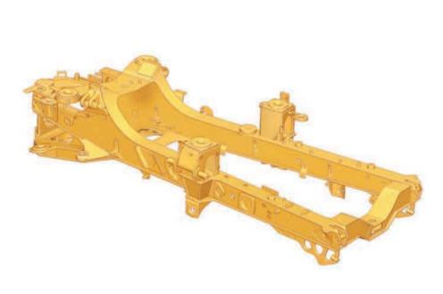
**Front Frame.** The front frame design features a large box-section, and wide, stiff frame beams to handle torque loads. The divergent frame design decreases stress in the hitch area and optimizes suspension geometry. The frame has been designed to make maximum use of robotic welding for increased durability.
