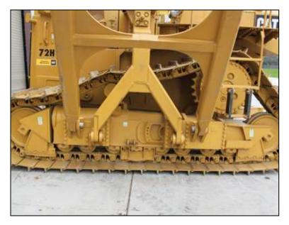
The 72H main frame is engineered to handle the unique demands of the pipelaying operation. The purpose-built steels side-skin plates reinforce the chasis, adding strength to the main case, center saddle and front cross member for outstanding durability.
