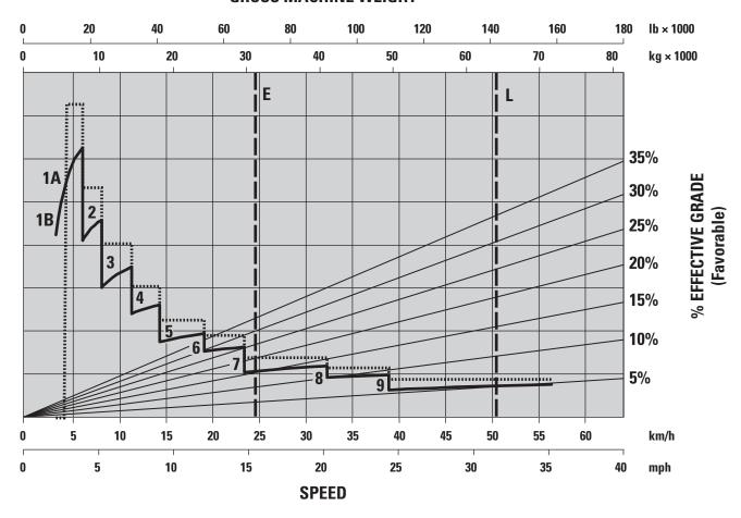
1A – 1st Gear (Converter Drive)
