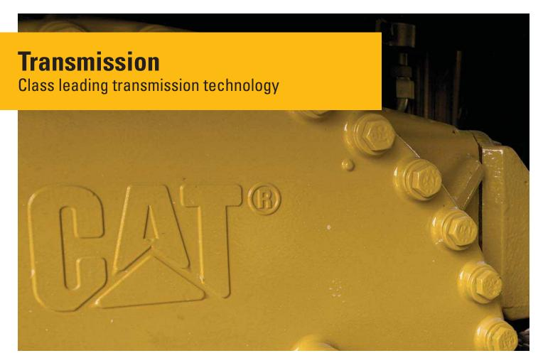
The new Cat High Density Power Shift (HDPS) nine-speed forward two-speed reverse transmission, designed specifically for Articulated Trucks, features Advanced Productivity Electronic Control Strategy (APECS) and Electronic Clutch Pressure Control (ECPC) which deliver smooth gear changes with improved acceleration and higher productivity.
