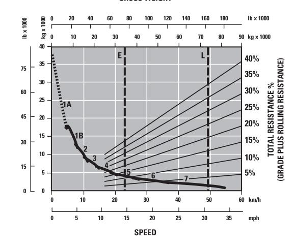
1A – 1st Gear (Converter Drive)
