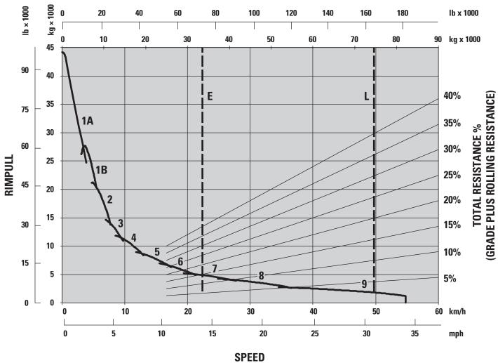
1A – 1st Gear (Converter Drive)
