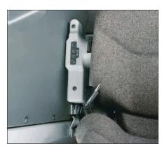
**14 Electrohydraulic Hoist Lever.**Is fingertip actuated and provides low impact body-down snubbing.
