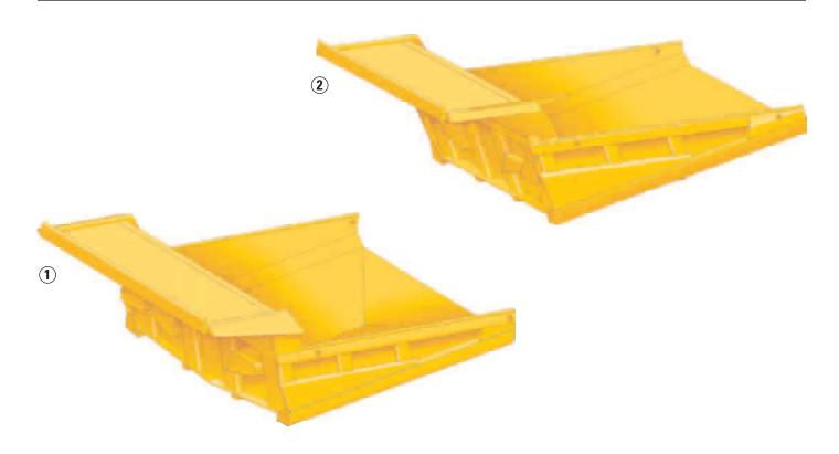
**Design.** 769D bodies are designed to handle a variety of material densities. Maximum payload is reached in three to five passes from a matched Cat loader in 1700 kg/m³ material and higher.
