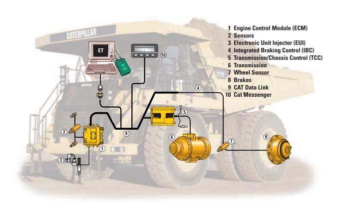
**Cat Data Link.** Electronically integrates machine computer systems to optimize overall power train performance, increase reliability and component life, and reduce operating costs. All control modules communicate via the Cat Data Link and work together as an integrated system to maximize production efficiency and extend component life.
