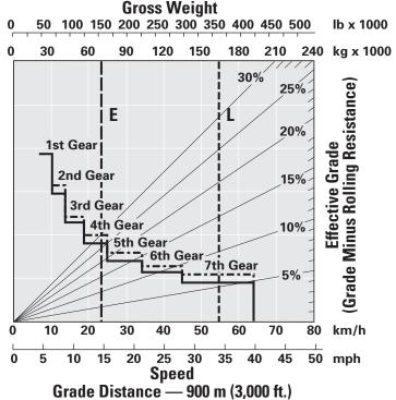
With ARC Only ---- ARC and Engine Brake
