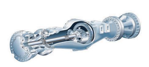
**Front Axle.** Is rigidly mounted to the frame to support the weight of the compactor, internal torque loads and external loads applied during compacting and dozing operations.
