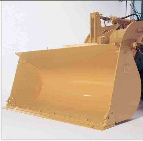
**Ground Engaging Tools.** Ground engaging tools include hardened steel cutting edges, choice of short or long teeth and a variety of tooth adapters. These tools optimize performance, improve load retention and extend the useful life of Caterpillar buckets.
