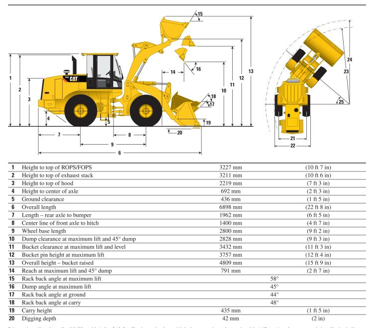
Dimensions listed are for 924Hz with 1.8  $\text{m}^3$  (2.3  $\text{yd}^3$ ) pin-on bucket with bolt-on cutting edge, cab with A/C, optional counterweights, limited slip axles, heavy duty rear brakes, additional guarding, sound suppression, work tool, 80 kg (176 lb) operator and Michelin 20.5 R25 L3 XHA tires.
