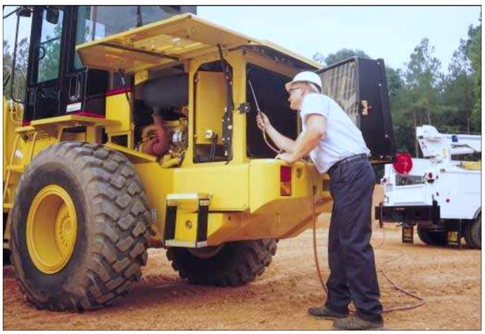
Easy, Wide Open Access. Gull-wing engine enclosure doors with pneumatically-assisted lift cylinders effortlessly lift up for exceptional access to major power train components. All filters and service points are within easy reach.
