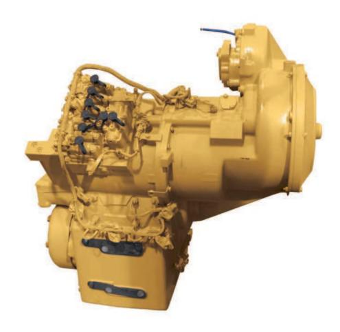
**Traction Control System.** The Caterpillar exclusive Traction Control System traction aid (attachment) has been improved for G Series II. Sensors and connectors have been upgraded for longer life. A new lighted cab switch indicates when the TCS system is "on."
