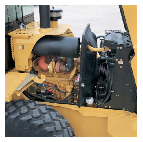
**Turbocharged, ATAAC.** Turbocharging packs dense air into the cylinders for more complete combustion and lower emissions. Air-to-air aftercooling (ATAAC) provides a separate cooling system for intake manifold air. The ATAAC system reduces smoke and emissions by providing cooler inlet air for more efficient combustion.
