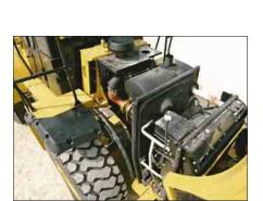
A single mechanical lift cylinder with manual back-up opens the hood. The tilting hood provides excellent access to the engine compartment, and if necessary, the entire hood can be removed with the built-in lift points. With the hood closed, quick checks of engine oil level and the coolant sight gauge can be completed through the side service doors.
