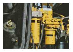
**Electric Priming Pump.** An electric fuel priming pump located on the primary fuel filter base eliminates the need to pre-fill or manually prime filters after a change, eliminating engine contamination.
