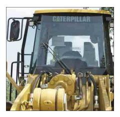
**Cab.** The entire operator station can be removed in about 45 minutes and is easy to re-attach. Quick disconnects are used so no wires need to be cut and no refrigerant is lost.
