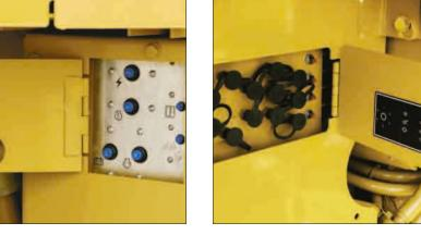
**Remote Pressure Taps.** Pressure taps for the steering and hydraulic systems, transmission (optional) and brakes are grouped behind an access panel just below the right-side service platform.
