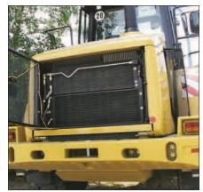
**Cooling System.** Access for clean-out and maintenance is outstanding. The perforated and corrugated grill minimizes debris build-up and swings out for easy cleaning and access to the cooling cores. The full-width air conditioning condenser and oil cooler cores swing out 45° to allow easy cleaning of the rear radiator face. Panels on either side provide access to the front face of the radiator and ATAAC cores for easy cleaning.
