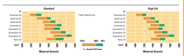
In accordance with SAE J818, these data consider the bucket load to be equal to half of the static tipping load at full turn.
