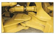
**Spread Hitch**. The distance between the upper and lower hitch plates is important for machine performance and component life. The Cat spread hitch design provides excellent load distribution and bearing life. Both the upper and lower hitch pins pivot on double tapered roller bearings – improving durability by distributing both vertical and horizontal loads over a larger surface area. The wide opening also provides excellent service access.
