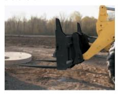
**Forks.** From pallet forks up through specialized logging arrangements, loader forks are available for a wide range of jobs.
