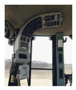
**CONTROLS.** The main control panel on the 962H is located high on the right ROPS post - keeping everything within reach of the operator while maintaining visibility to the ground. Keeping all switches and controls conveniently placed allows better efficiency and improved productivity all while minimizing operator fatigue.
