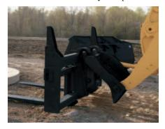
**Quick Couplers.** Quick couplers provide unmatched versatility for wheel loaders. The hydraulic model allows an operator to change attachments in seconds without leaving the cab. On the manual model, the operator must lock the pins.
