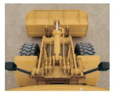
**Linkage.** The 962H linkage is a singletilt Z-bar design. Z-bar linkage generates excellent breakout force and good rack back angle for better bucket loading and load retention.
