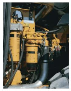
**ELECTRIC PRIMING PUMP.** An electric fuel priming pump located on the primary fuel filter base eliminates the need to pre-fill or manually prime filters after a change, eliminating engine contamination.
