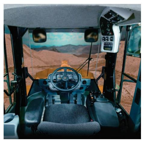
Command Control Steering. Command Control Steering is a load-sensing system that links the steering wheel and frame angle positions to provide the proper amount of steering control. The speed the machine turns is proportional to the steering wheel position. Less than 6 lb (26 N) steering effort is required by the operator, regardless of conditions. Full machine articulation is accomplished with a  $\pm 70^{\circ}$  turn of the
