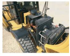
**ENGINE COMPARTMENT ACCESS.** The non-metallic hood on the 962H has been redesigned and restyled from previous models. Side and top panels are stronger due to more robust reinforcement ribs - the change in contour also adds to rigidity of the hood.
