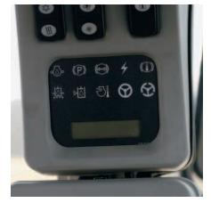
Caterpillar Monitoring System. The 962H is equipped with the Cat Monitoring System (CMS) that keeps watch over the health of your loader. CMS monitors critical engine system functions and will derate the engine to protect itself from damage if needed. Depending on which of the following six critical conditions arise, the CMS monitor or front panel will display warning lights and sound audible alarms.
