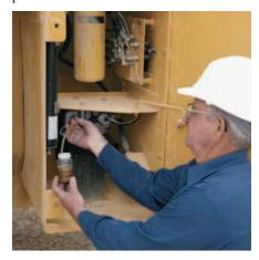
**S•O•S SERVICES.** Sampling valves on the 962H allow quick access to engine, transmission and hydraulic oils for S•O•S analysis. Oil change intervals and other services can be optimized according to your work schedule, reducing downtime and managing expenses.
