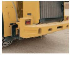
**Counterweight.** The one-piece counterweight is integrated into the 962H design and styling. This 3084 lb (1399 kg) counterweight incorporates the rear lights into the top of the structure.
