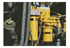
**Electric Priming Pump.** An electric fuel priming pump located on the primary fuel filter base eliminates the need to pre-fill or manually prime filters after a change, eliminating engine contamination.
