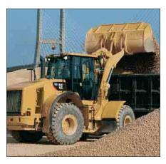
The standard programmable automatic kick-outs provide flexibility and productivity for precise load and dump target heights. Tilt, lift and return-to-dig kickouts are set by positioning the bucket or work tool and setting a rocker switch in the cab.
