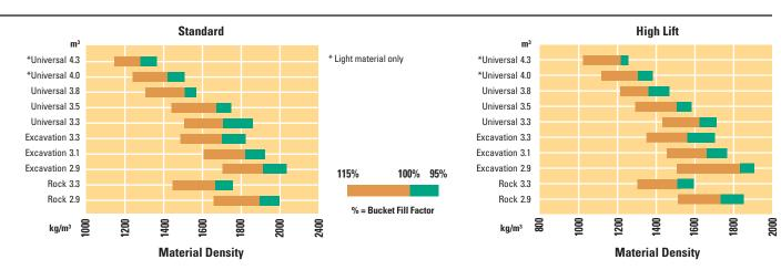
In accordance with SAE J818, these data consider the bucket load to be equal to half of the static tipping load at full turn.
