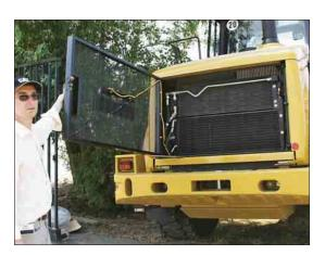
**Cooling System.** Access for clean-out and maintenance is outstanding. The perforated and corrugated grill minimizes debris build-up and swings out for easy cleaning and access to the cooling cores. The full-width air conditioning condenser and oil cooler cores swing out 45° to allow easy cleaning of the rear radiator face. Panels on either side provide access to the front face of the radiator and ATAAC cores for easy cleaning.
