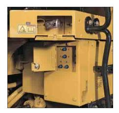
**Electric Service Center.** Batteries, relay panel and an optional tool box are conveniently located below the left-side access platform. The engine shutdown switch is housed with the relay panel. A compartment integrated into the access platform contains the hood tilt actuation switch, battery disconnect switch and optional jump-start receptacle.
