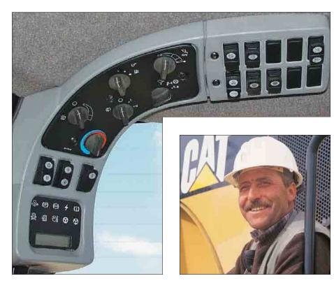
**Controls.** The main control panel on the 966H is located high on the right ROPS post – keeping everything within reach of the operator while maintaining visibility to the ground. Keeping all switches and controls conveniently placed allows better operator efficiency and improved productivity, while minimizing operator fatigue.
