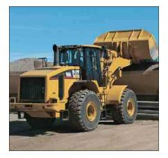
The standard programmable automatic kick-outs provide flexibility and productivity for precise load and dump target heights. Tilt, lift and return-to-dig kickouts are set by positioning the bucket or work tool and setting a rocker switch in the cab.
