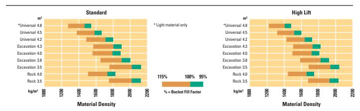
In accordance with SAE J818, these data consider the bucket load to be equal to half of the static tipping load at full turn.
