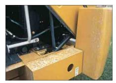
A single mechanical lift cylinder with manual back-up opens the hood. The tilting hood provides excellent access to the engine compartment, and if necessary, the entire hood can be removed with the built-in lift points.
