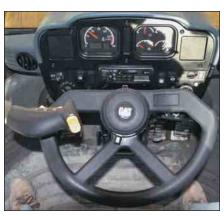
Full machine articulation is accomplished with a  $\pm 70^{\circ}$  turn of the wheel – versus two to three 360° turns of a conventional steering wheel. The Command Control Steering wheel contains the forward/ neutral/reverse switch and the upshift/ downshift button – allowing the left hand to remain on the steering wheel at all times. The CCS column inclines 35° and the telescopic change is up to 100 mm.
