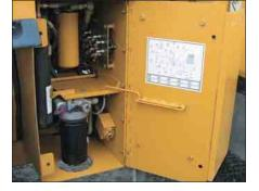
**Hydraulic Service Center.** Transmission oil and hydraulic oil filters are located in the Hydraulic Service Center, behind the hinged, right-side access ladder. The hydraulic oil tank can be drained from this location using the access port.
