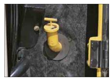
With the hood closed, quick checks of engine oil level and the coolant sight gauge can be completed through the side service doors.
