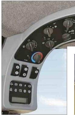
**Controls.** The main control panel on the 966H is located high on the right ROPS post – keeping everything within reach of the operator while maintaining visibility to the ground. Keeping all switches and controls conveniently placed allows better operator efficiency and improved productivity, while minimizing operator fatigue.
