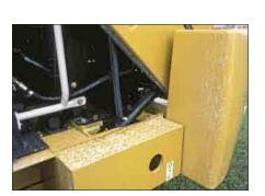
A single mechanical lift cylinder with manual back-up opens the hood. The tilting hood provides excellent access to the engine compartment, and if necessary, the entire hood can be removed with the built-in lift points.
