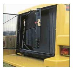
**Cooling System.** Access for clean-out and maintenance is outstanding. The perforated and corrugated grill minimizes debris build-up and swings out for easy cleaning and access to the cooling cores. The full-width air conditioning condenser and oil cooler cores swing out 45° to allow easy cleaning of the rear radiator face. Panels on either side provide access to the front face of the radiator and ATAAC cores for easy cleaning.
