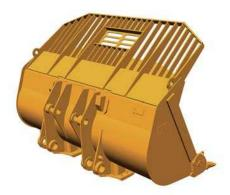
• General Purpose Landfill bucket – has a capacity of 4.9 m³ (6.4 yd³) and can be equipped with an optional trash rack for dozing lightweight materials. This bucket is designed for easy loading in stockpile or hard bank materials. Adding the trash rack helps prevent material from spilling over the top and increases dozing capacity by 52%.
