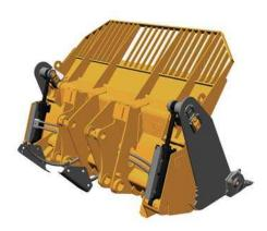
• Multi Purpose Landfill bucket – has a capacity of 4.6 m<sup>3</sup> (6.0 yd<sup>3</sup>) and can greatly expand the 973D's versatility. It can act as a typical bucket for loading trucks, dozing waste or digging. It can also instantly change into a dozer-type blade for spreading cover material, or it can sort material with the ability to clamp on to debris. By adding the trash rack to this bucket, its capacity to doze and load material increased 53%.
