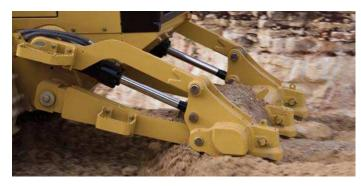
Ripper – A 3-shank parallelogram ripper facilitates working in frozen ground and hard materials like asphalt, rocky ground and hard clay. Ripper shank options are available to help improve ripping productivity.
