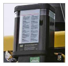
**Autolube.** Reduce time spent on daily maintenance and downtime for unplanned repairs due to inadequate greasing with the optional Caterpillar Automatic Lubrication System. Precise lubrication of pins and bushings at specific intervals decreases component wear and reduces ground contamination from excessive greasing.
