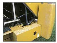
The tilting hood provides excellent access to the engine compartment, and if necessary, the entire hood can be removed with the built-in lift points.
