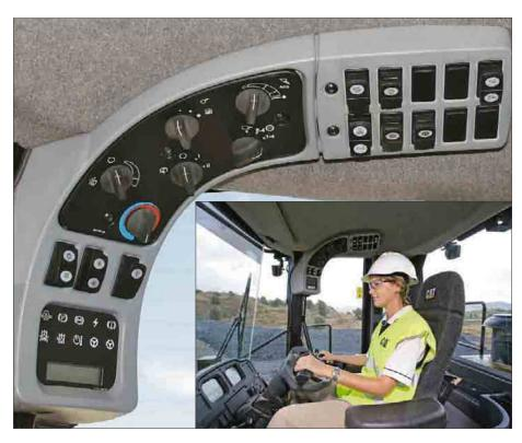
**Controls.** The main control panel on the 980H is located high on the right ROPS post – keeping everything within reach of the operator while maintaining visibility to the ground. Keeping all switches and controls conveniently placed allows better operator efficiency and improved productivity, while minimizing operator fatigue.
