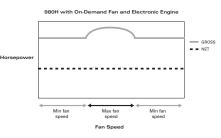
**Constant Net Horsepower.** The engine automatically compensates for parasitic loads, like the fan and air conditioner, to maintain a consistent level of productivity.
