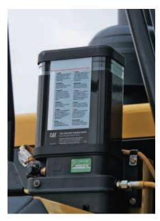
**Autolube.** The optional Caterpillar Autolube System provides precise, automatic lubrication of pins and bushings – during loader operation. Automatic lubrication reduces time spent on daily maintenance and downtime for unplanned repairs due to inadequate greasing – improving productivity.
