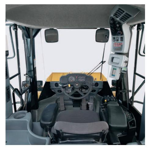
**Ease of Operation.** Command Control Steering is a load-sensing system that links the steering wheel and frame angle positions to provide the proper amount of steering control. The speed the machine turns is proportional to the steering wheel position. Less than 26 N (6 lb) steering effort is required by the operator, regardless of conditions. Full machine articulation is accomplished with a  $\pm 70^{\circ}$  turn of the wheel – versus two to three 360° turns of a conventional steering wheel.
