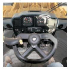
**Command Control Steering.** Reduce steering movements by a factor of 14 with Command Control Steering as compared to conventional steering. A conventional steering wheel requires two to three  $360^{\circ}$  turns to complete one turn of the loader – the Command Control wheel moves  $\pm 70^{\circ}$  with only 26 N (6 lb) steering pressure to complete a turn – reducing operator fatigue.
