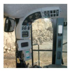
**Controls.** The main control panel on the 980H is located high on the right ROPS post – keeping everything within reach of the operator while maintaining visibility to the ground. Clear graphical symbols make the switches easy to understand and operate.
