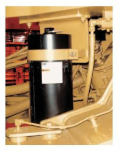
**Ride Control.** The optional Ride Control System improves ride, performance and load retention when traveling over rough terrain. Operators gain confidence moving at higher speeds in load and carry operations decreasing cycle time and increasing productivity.
