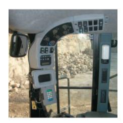
**Integrated Systems.** The Caterpillar Monitoring System (CMS) tracks critical machine systems to alert the operator to potential need for service. Three levels of warning allow the operator to assess the situation more accurately. CMS is tied to the engine, transmission, hydraulics and brakes – connecting all major systems allows the loader to work as a fully integrated system – from the linkage to the engine.
