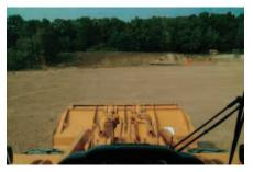
**Visibility.** The 980H provides excellent visibility to both the front and rear of the machine. Distortion-free flat glass stretches to the floor of the cab for excellent visibility to the bucket. Wet-arm wipers on both front and back keep the windows clean in any condition. The cab roof has channels that direct rain off the corners of the cab keeping windows clear. An overhang on all sides protects the operator from glare.
