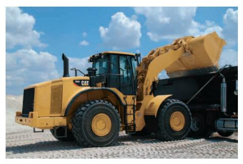
**Aggregate Autodig.** Well-received by both experienced and novice operators, the optional Aggregate Autodig is available to automate the loading process. Operators get consistently full payloads without touching the controls.
