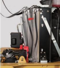
Ground level access, right-side-of-machine service, and visual indicators are just a few of the features that make Cat machines easier and less expensive to service than the competition. The CS44 and CP44 also feature a maintenance-free articulation hitch and a tilting oil cooler for greater service access.
