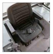
**Seat.** A comfortable suspension seat is able to be adjusted fore and aft for greater operator comfort. Arm rests also help provide comfort for all day operation. Wide 76 mm seat belt is standard.
