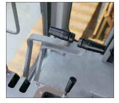
**Directional Controls.** Steering and transmission controls are located conveniently to the operator's left for comfortable operation.
