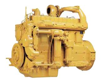
**3306 Diesel Engine.** The Caterpillar® 3306 is a six-cylinder, four stroke diesel. The large displacement allows lower engine speeds for reduced stresses and increased engine life.
