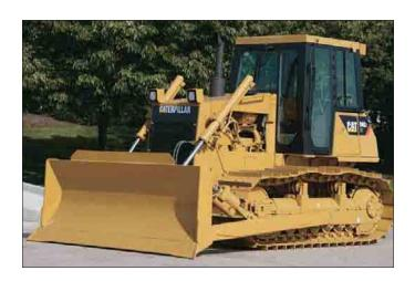
**Torque Divider.** The torque divider arrangement is a Caterpillar exclusive that provides high torque multiplication when under load with direct drive efficiency when completing lower engine load functions such as backfilling trenches or spreading material.
