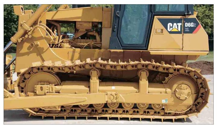
**Roller Frames.** The track roller frame is a reinforced box section construction with seven lifetime lubricated track rollers per side and outside mounted carrier rollers, two per side.
