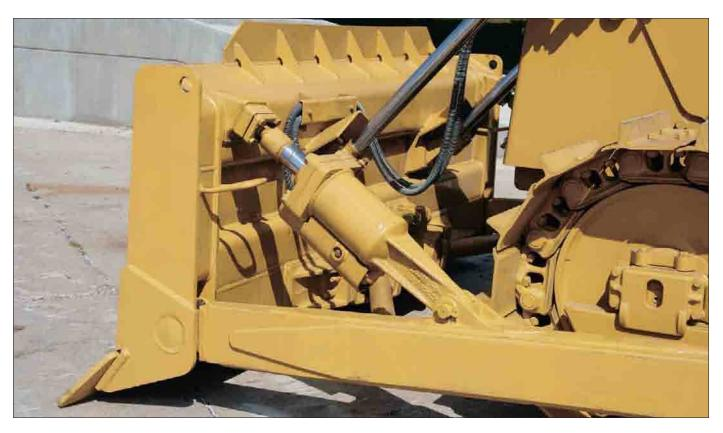
**Bulldozers.** All blades feature a strongbox-section design that resists twisting and cracking. Blades are made of Cat DH-2<sup>TM</sup> steel that has high tensile strength and stands up to the most severe applications. Heavy moldboard construction and hardened bolt-on cutting edges and end bits add strength and durability.
