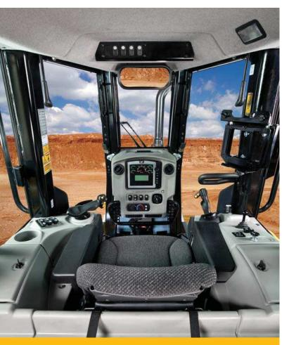
An isolation-mounted pressurized cab reduces dust entry, noise and vibration. Large glass panels provide excellent visibility. Intermittent wipers maximize visibility in poor weather conditions. Heating and air conditioning controls are conveniently located. Temperature control is automatic.
