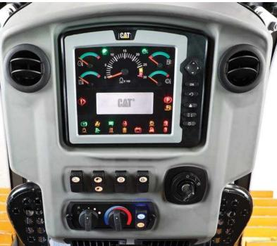
All controls are electro-hydraulic, which means precision and maneuverability. They are ergonomically designed for easy intuitive, comfortable and low effort operation. Blade response can be adjusted through the operator profile in the display.
