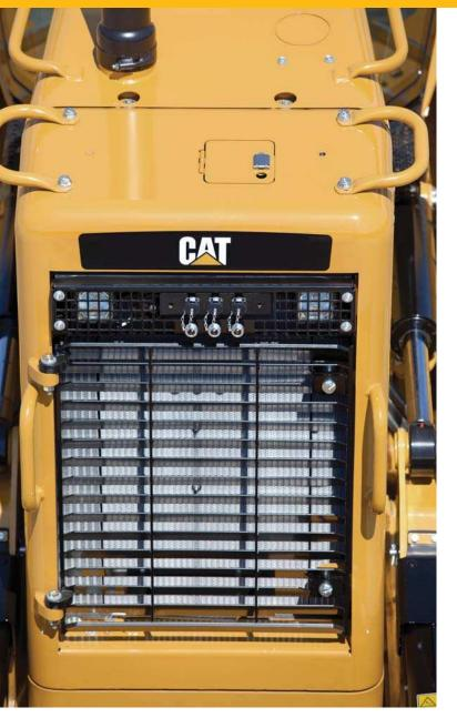
The engine radiator, Air To Air After Cooler (ATAAC), and hydraulic oil cooler are packaged in a single plane. Aluminum bar plate construction provides durability and allows for higher heat transfer and superior corrosion resistance. The standard cores feature 8.9 fins per inch (6.5 fins per inch for the Waste Handling Arrangement) to allow debris to pass through and reduce plugging concerns.
