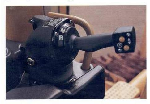
Tiller Bar Control System. The tiller bar control system allows for simultaneous comfortable, one-handed steering, direction and transmission control.
