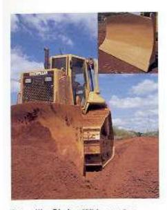
Caterpillar Blades. With superior moldboard and 4-cell structure design, Cat hulldozer blades hold up to the toughest job conditions. Our high-tensile strength blades resist torsional bending and deflection in tough applications.
