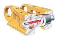
Rotating Bushing Track. Rotating Bushing Track is designed to extend system life and lower costs in highly abrasive low to moderate impact applications. RBT features bushings which rotate when in contact with the sprocket, greatly reducing bushing and sprocket wear. This design eliminates bushing turn maintenance expense and sprocket replacement costs.
