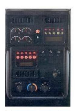
Dash. The instrument panel, with easy to read analog gauges and warning lamps, keeps the operator aware of any potential problems. All gauges and readouts are easily visible in direct sunlight. HVAC controls and veuts are conveniently located on the dash to provide climate control for the operator. Auto-shift and Auto-kickdown controls are located within easy reach of the operator. New footpads keep the operator stable and comfortable during side slope applications.
