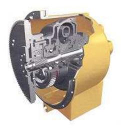
Torque Converter. The D6N single stage torque converter efficiently responds to changing load conditions by providing torque multiplication, therefore increasing drawbar power. It also provides protection to the drive train components by preventing shock loads in heavy dozing applications. This torque converter is efficiently matched to the power train components and provides the superior performance you need.
