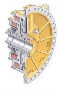
Transmission. The proven planetary powershift transmission features three speeds forward and three speeds reverse and utilizes large diameter, high capacity, oil cooled clutches. To maximize the life of the transmission, the planetary design distributes stress over multiple gears.
