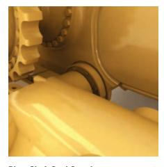
**Pivot Shaft Seal Guards.** The pivot shaft seal guards help prevent debris from entering and damaging the Duo-Cone® seals as well as protecting the bolts on the pivot shaft seal retainers.
