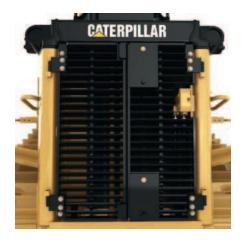
Hinged Radiator Guard. The hinged radiator guard protects the cooling system. It comes equipped with two quick release "T" handles for the center-opening guard, allowing easy access to the radiator for cleaning. Covers protect the handles from damage. Special hinge latches retain the guard in the open or closed positions.
