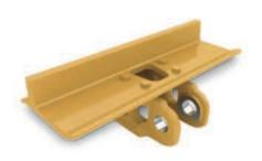
Trapezoidal Hole Track Shoes (D7R Series II). The trapezoidal hole track shoes reduce refuse packing within the track and reduces track chain tightening and accelerated pin and bushing wear. The trapezoidal holes relieve packing by allowing the sprocket to punch out dirt and debris.
