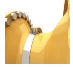
**Final Drive Seal Guards.** The final drive seal guards help prevent wire, nylon strapping, etc., from wrapping around and damaging the Duo-Cone seals. The outer guard is now stationary, thicker, and has increased hardness, all of which help prevent excessive wear from debris.
