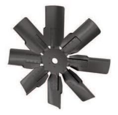
**Ejector Fan.** The ejector fan blade is designed with curved edges to help throw debris out radially. This helps prevent debris from clogging the radiator.
