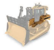
Additional Sealing. To help eliminate debris entry into areas of the machine additional sealing is provided. Key areas include: engine enclosures, platforms, hydraulic tank, ROPS support, battery box, striker bar box, and rear case opening.
