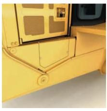
**Chassis Guards.** The chassis guards help protect the engine compartment by deflecting debris from rising upward along the chassis.
