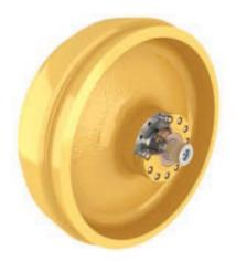
**Idler Seal Guards.** The idler seal guards help keep wire, fishing line, strapping, etc., from wrapping around and damaging the Duo-Cone seals.
