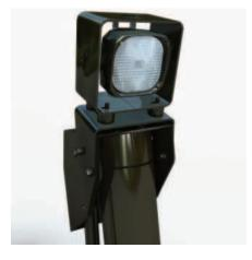
**Front Lights.** The front lights are mounted on top of the bulldozer lift cylinders allowing them to project light over the trash rack and keep the lights above the concentrated debris environment for longer service life.
