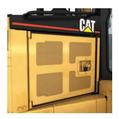
**Engine Enclosures.** The engine enclosures consist of perforated hood and side panels. The enclosures help prevent airborne materials from entering the engine compartment and help reduce radiator plugging, which can cause cooling system problems.
