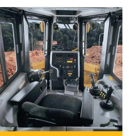
The D6T cab is designed for operator productivity, safety and comfort. An isolation-mounted, pressurized cab reduces noise and vibration. Large single-pane windows offer excellent visibility. The low rear window enables excellent rearward visibility and lets the operator see the ripper tip. The tapered hood, notched fuel tank, and narrow single-shank ripper carriage give the operator a clear line of sight to front and rear work areas.
