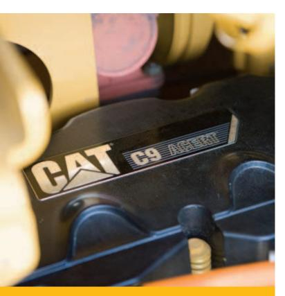
The D7E electric drive train is powered by a 235 hp Cat C9.3 engine with ACERT<sup>™</sup> Technology. The engine utilizes a proven common rail fuel system for improved efficiency and fuel economy. Featuring the latest in Cat emissions reduction technologies, this engine meets U.S. EPA Tier 3, EU Stage IIIa and Japan MLIT Step 3 emissions regulations.
