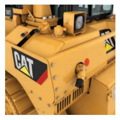
**Fast Fuel System.** The optional fast fuel system, with positive fuel shut-off to prevent fuel spillage, can decrease downtime.
