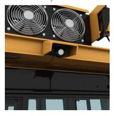
**Rear Vision Camera.** An attachment WAVS rear vision camera is available to provide additional visibility to the standard mirrors.
