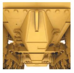
**Crankcase (belly) Guards.** The crankcase (belly) guards serve a dual purpose. They help prevent contact damage to vital power train components, and help keep debris out of the power train compartments.
