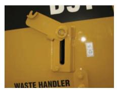
**Clean-Out Slots.** Clean-out slots are available to help keep the radiator core clear from debris. Machines equipped with clean-out slots are able to be manually cleaned to help keep your machine running trouble free.
