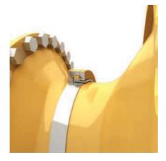
**Final Drive Seal Guards.** The final drive seal guards help prevent wire, nylon strapping, etc., from wrapping around and damaging the Duo-Cone seals. The outer guard is now stationary, thicker, and has increased hardness, all of which help prevent excessive wear from debris.
