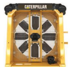
**Hydraulic Reversing Fan.** The fan system automatically reverses the fan at preset intervals, purging debris from the radiator and engine compartment. The operator can manually purge at anytime. The fan is controlled by the engine electrical control module.
