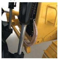
**Tilt Cylinder Lines Guards.** The tilt cylinder lines guards help protect hydraulic lines from contact damage, while maintaining hose flexibility.
