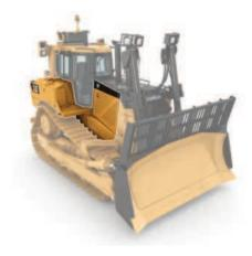
**Additional Sealing.** To help eliminate debris entry into areas of the machine additional sealing is provided. Key areas include: engine enclosures, platforms, hydraulic tank, ROPS support, battery box, striker bar box, and rear case opening.
