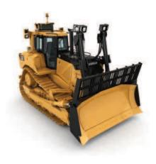
Black Painted Hood, Cylinders, and Back of Blade. The black painted hood, cylinders, and back of blade reduces glare from lights while operating at night and while operating in direct sunlight.
