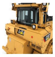
Hydraulic and Fuel Tank guard. The hydraulic and fuel guard helps protect implement hydraulic oil tank, battery box and fuel tank.
