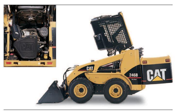
**Service Access.** The rear service door opens 90 degrees for easy access to both sides of the in-line mounted engine.
