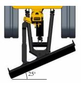
Angle Blade Positioning. The angle blade can be positioned straight ahead or angled up to 25 degrees to the left or right reducing the number of times required to back-up and reposition when backfilling thus reducing operation time.
