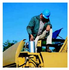
**Capsule Filter.** The hydraulic return filter, a capsule filter, is situated outside the hydraulic tank. This filter prevents contaminants from entering the system when hydraulic oil is changed and keeps the operation clean.
