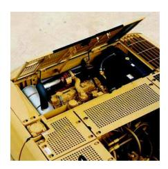
**Engine Inspection.** Engine can be accessed from the upper structure or from under the machine. The engine and pump compartment are separated by a steel wall.
