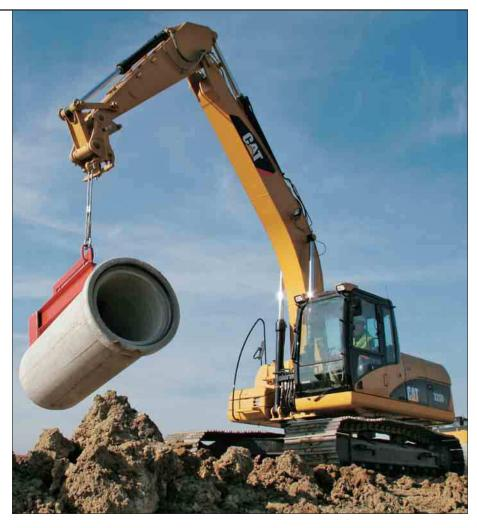
**Auxiliary Hydraulic Valve.** The auxiliary valve is standard on the 320D L. Control Circuits are available as attachments, allowing for operation of high and medium pressure tools such as shears, grapples, hammers, pulverizers, multi-processors and vibratory plate compactors.
