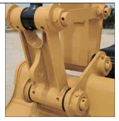
**Bucket Linkage.** The power link improves durability, increases machinelifting capability in key lifting positions and with the integrated lift-eye it is easier to use than compared to the previous power link. The lift eye also gives you the optimum lift performance. It allows you to lower the load point, which maximizes the use of the boom cylinders.
