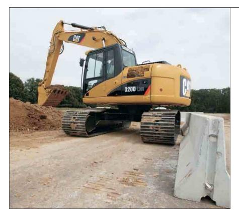
**Reduced Radius.** The tail swing of this machine has been reduced where the back end of the machine won't extend beyond the length of the tracks. The tail swing is just 2000 mm as compared to the 2750 mm on the 320D. When rotated 90 degrees and working over the side, just 600 mm hangs over the side. This allows the 320D LRR to work well in road construction applications and other space restricted areas.
