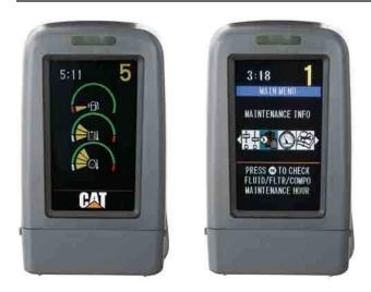
**Monitor.** The monitor is a full color Liquid Crystal Display that gives you vital operating and performance information, alerts in text, all in a simple, east to navigate format.
