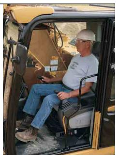
**Comfort.** The cab on the 321D LCR is a comfortable place to work, with low sound levels, good visibility and convenient access to switches and controls.
