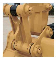
**Bucket Linkage.** The power link improves durability, increases machine-lifting capability in key lifting positions and with the integrated lift-eye it is easier to use than compared to the previous power link. The lift eye also gives you the optimum lift performance. It allows you to lower the load point, which maximizes the use of the boom cylinders.
