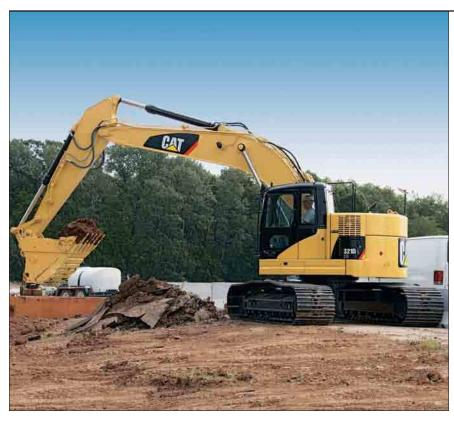
Compact Radius. The 321D LCR features a compact radius design, which makes it ideal for working in space restricted areas such as: close to buildings, road construction – limiting lane closures or logging roads. The tail swing is just 1680 mm as compared to the 2750 mm on the 320D. When rotated 90 degrees and working over the side, a minimal amount of counterweight extends beyond the track width.
