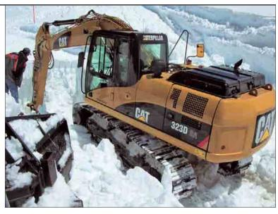
**Undercarriage.** The 323D SA undercarriage consists of two 325D track roller frames. It provides the best choice when an extra rugged undercarriage is important while maintaining ease of transport.
