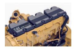
**Diesel Engine.** The Caterpillar C18, with ACERT technology, is a 18.1 liter, six-cylinder, 382 kW (513 hp) engine with mechanically actuated electronic fuel injection (MEUI) and overhead camshaft. ACERT technology provides outstanding engine performance through advanced electronic control, precision fuel delivery, and refined air management.
