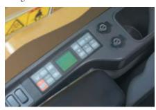
**Consoles.** Redesigned consoles feature a simple, functional design to reduce operator fatigue, ease of switch operation and excellent visibility. Both consoles have attached armrests and allow the height of the armrests to be adjusted.
