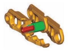
**Track.** The 385C L comes standard with the new grease lubricated track called GLT4. The track links are assembled and sealed with grease to decrease internal bushing wear, reduce travel noise and extend service life lowering operating costs.
