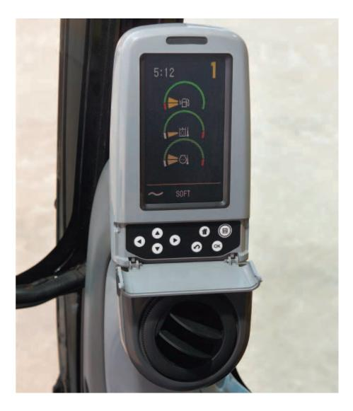
**Monitor Display Screen.** The monitor is a full color 400 × 234 pixels Liquid Crystal Display (LCD) graphic display.
