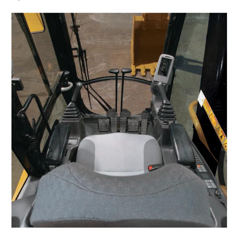
**Cab Design.** The work station has been designed to be spacious, quiet and comfortable. Operator comfort, and a high level of visibility assure productivity throughout the entire workday. The monitor and switches are conveniently located for easy access and visibility.
