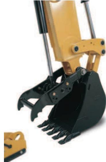
**Thumb Mounting.** Thumb mounting provisions are standard on every Cat Backhoe Loader for added machine versatility. Hydraulic thumbs are available factory-installed.
