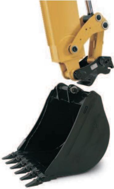
*Soil Excavation Bucket with Coupler*
