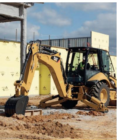
The 416E has a load-sensing, closed center hydraulic system, which closely matches power and flow to the demand needed by the implements. So whether you're in full trenching mode, or delicately digging around services, you are in control. In applications such as production trenching, speed is important and the system will match the flow needed to get the job done quickly and efficiently. The load-sensing hydraulic system also delivers:
