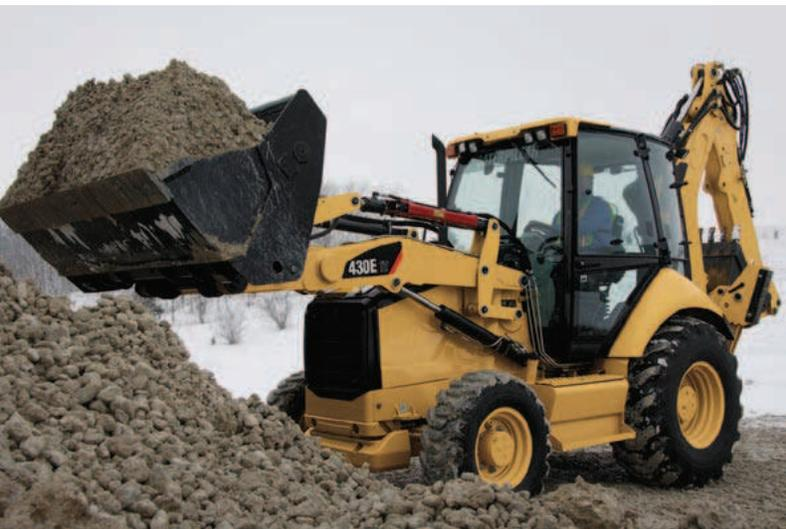
Caterpillar offers a choice of single tilt or integrated toolcarrier (IT) loader linkage to suit your application requirements. The IT loader controls provide single lever proportional control and fine modulation of the hydraulic work tools. A thumb roller operates auxiliary hydraulic functions such as the multi purpose bucket on the IT machines.
