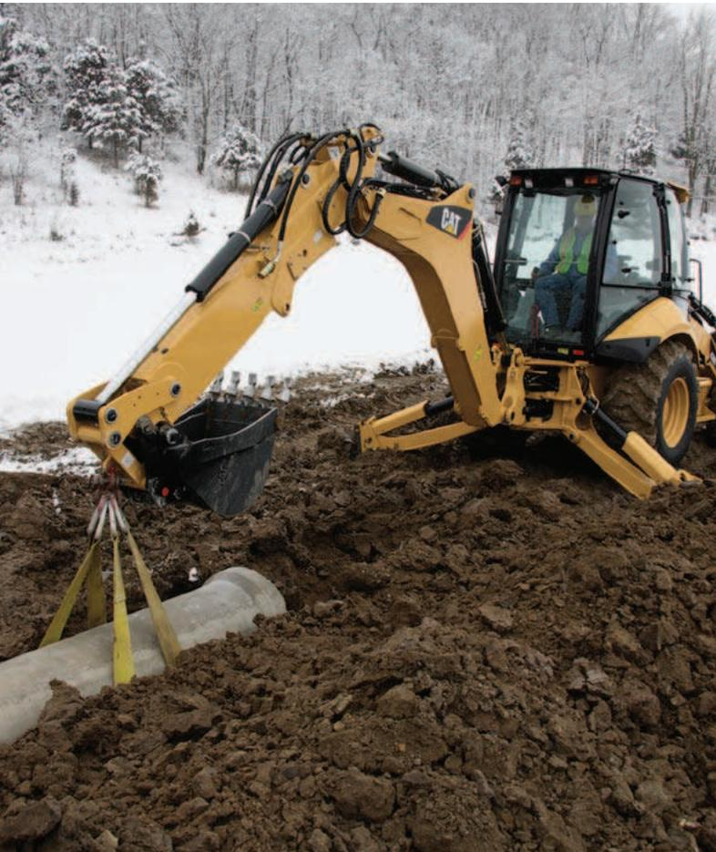
The 430E has a load-sensing, closed center hydraulic system, which closely matches power and flow to the demand needed by the implements. So whether you're in full trenching mode, or delicately digging around services, you are in control. In applications such as production trenching, speed is important and the system will match the flow needed to get the job done quickly and efficiently. The load-sensing hydraulic system also delivers:
