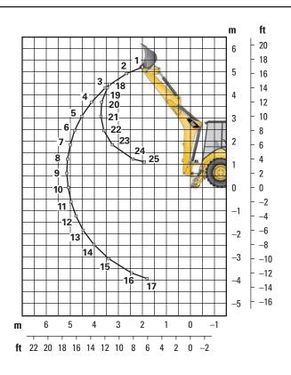
Lift Capacities are over-end values. Machine equipped with 4WD, OROPS, 1.00 m<sup>3</sup> (1.31 yd<sup>3</sup>) general purpose bucket, and 116 kg (255 lb) counterweight. Extendible stick includes 488 kg (1,075 lb) counterweight.
