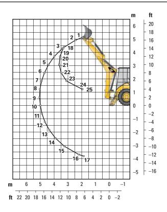
Lift Capacities are over-end values. Machine equipped with 4WD, OROPS, 1.00 m<sup>3</sup> (1.31 yd<sup>3</sup>) general purpose bucket, and 116 kg (255 lb) counterweight. \*Indicates lift capacity is stability limited.
