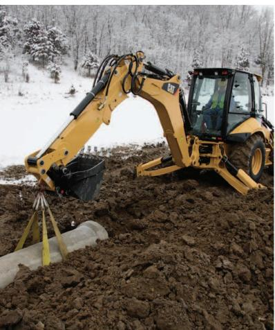
The 430E has a load-sensing, closed center hydraulic system, which closely matches power and flow to the demand needed by the implements. So whether you're in full trenching mode, or delicately digging around services, you are in control. In applications such as production trenching, speed is important and the system will match the flow needed to get the job done quickly and efficiently. The load-sensing hydraulic system also delivers:
