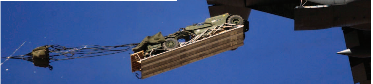
613C II Scraper executing a Low Velocity Air Drop from a C-130.
