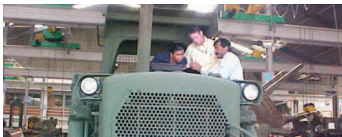
Caterpillar Kuwait dealer, Al Bahar, executing SLEP repairs on D7G
