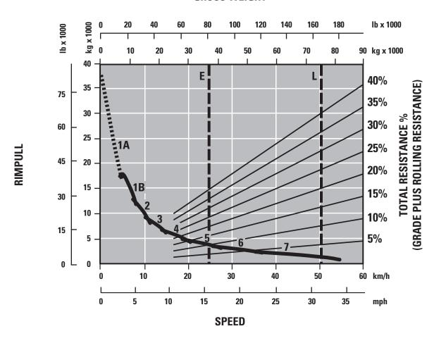
1A – 1st Gear (Converter Drive)
