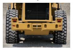
**Counterweight.** The two-piece counterweight is integrated into the 938H design and provides added protection for the lights by incorporating them into the top of the structure.
