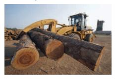
**Forks.** Logging, Millyard and Pallet Forks are available for forestry and material handling applications.
