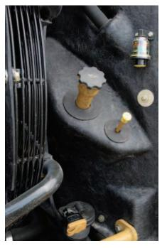
With the hood closed, quick checks of the engine oil level, coolant site gauge and air inlet indicator can be completed through the side service door. **ECOLOGY DRAINS.** Engine, transmission and hydraulic oils can be easily drained with standard-equipment ecology drains. An axle oil ecology drain is optional.
