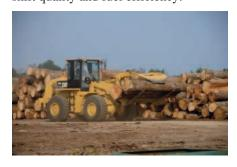
RIDE CONTROL. The optional Ride Control System improves ride, performance and load retention when traveling over rough terrain. Operators gain confidence moving at higher speeds in load and carry operations decreasing cycle times and increasing productivity.
