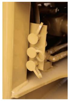
**REMOTE PRESSURE TAPS.** Pressure taps for key systems are grouped and centrally located throughout the machine and help facilitate quick diagnostics.
