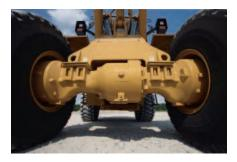
**NEW! DIFFERENTIAL LOCK.** Maximize productivity with the new hydraulic locking front differential. This standard feature provides operators with the confidence to maneuver through poor underfoot conditions with 'on the fly' engagement.
