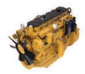
**Cat C6.6 ACERT.** The Cat C6.6 is a 6.6 liter (403 in³) displacement, in-line six cylinder engine. The C6.6 utilizes ACERT Technology, a series of Caterpillar engineered innovations that provides advanced electronic control, precise fuel delivery and refined air management, resulting in outstanding performance and lower emissions.
