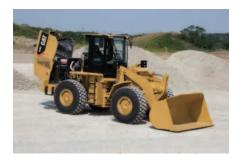
A single mechanical lift cylinder with manual back-up opens the hood. The tilting hood provides excellent access to the engine and cooling compartments and if necessary, the entire hood can be removed with the built-in lift points.
