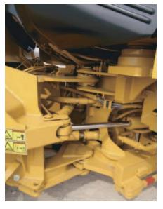
Spread Hitch. The distance between the upper and lower hitch plates is an important contributor to machine performance and component life. The Caterpillar spread hitch design provides excellent load distribution and bearing life. Both the upper and lower hitch pins pivot on double tapered roller bearings improving durability by distributing both vertical and horizontal loads over a larger surface area. The wide opening also provides excellent service access.
