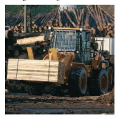
**Lumber and Log Forks.** Lumber and log forks are ideal for a wide range of jobs loading, decking and sorting lumber, logs or palletized material.
