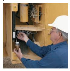
**S•O•S SERVICES.** Sampling valves on the 950H allow quick access to engine, transmission and hydraulic oils for S•O•S analysis. Oil change intervals and other services can be optimized according to your work schedule, reducing downtime and managing expenses.
