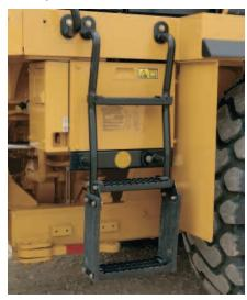
**ENTRY AND EXIT.** A ladder with self-cleaning steps keeps debris build-up to a minimum. The ladder is at a 5° forward incline for easy entry and exit.
