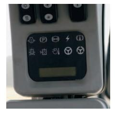
Caterpillar Monitoring System. The 950H is equipped with the Cat Monitoring System (CMS) that keeps watch over the health of your loader. CMS monitors critical engine system functions and will derate the engine to protect itself from damage if needed. Depending on which of the following six critical conditions arise, the CMS monitor or front panel will display warning lights and sound audible alarms.
