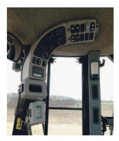
**CONTROLS.** The main control panel on the 950H is located high on the right ROPS post - keeping everything within reach of the operator while maintaining visibility to the ground. Keeping all switches and controls conveniently placed allows better efficiency and improved productivity all while minimizing operator fatigue.
