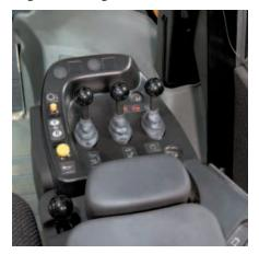
**Seat.** The Cat C-500 Series Comfort air suspension seat, standard in the 950H, is built strong and durable and is 6-way adjustable to accommodate all-sized operators. The cast one-piece back and seat pan prevent protrusions under the cushions. The seat features an automotive-style lumbar support for maximum comfort. The right hand armrest with integrated implement controls adjusts for comfortable, convenient operation. A heated seat option is available for additional comfort.
