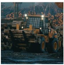
Forestry Applications. The Forest Machine Arrangement provides Ride Control, a heavy-duty tilt cylinder and an additional counterweight for use in forestry and logging applications. Specially-designed work tools for forestry applications can be factory-installed.
