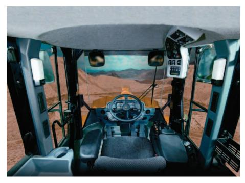
Command Control Steering. Command Control Steering is a load-sensing system that links the steering wheel and frame angle positions to provide the proper amount of steering control. The speed the machine turns is proportional to the steering wheel position. Less than 6 lb (26 N) steering effort is required by the operator, regardless of conditions. Full machine articulation is accomplished with a ±70° turn of the wheel - versus two to three 360° turns of a conventional steering wheel.
