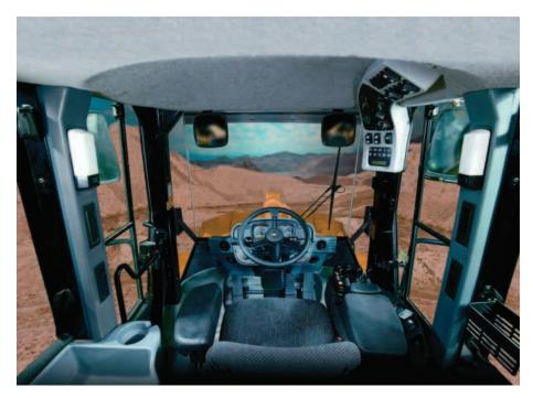
The Command Control Steering wheel contains the forward/neutral/reverse switch and the upshift/downshift button – allowing the left hand to remain on the steering wheel at all times. Implement controls are integrated into the right armrest so they move with the operator.
