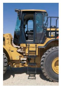
**ENTRY AND EXIT.** A ladder with self-cleaning steps keeps debris build-up to a minimum. The ladder is at a 5° forward incline for easy entry and exit.
