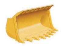
Rock Buckets. Rock buckets are designed for face or bank loading in mining or quarry applications. The straight-edge rock bucket provides higher breakout force and increased dump clearance. The spade-edge rock bucket offers increased penetration in certain applications.
