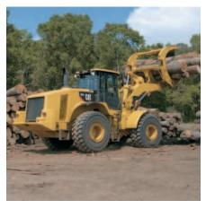
**Forestry Applications.** The Forest Machine Arrangement provides Ride Control, a heavy-duty tilt cylinder and an additional counterweight for use in forestry and logging applications.
